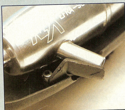
After having seen stingers break off during a race we know why Chad uses the guard.
