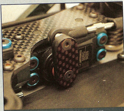
For added rigidity Chad fits his servo horn with a carbon fiber brace.
