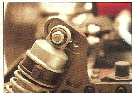
Chad sticks with the middle two holes on both of the shock towers.
